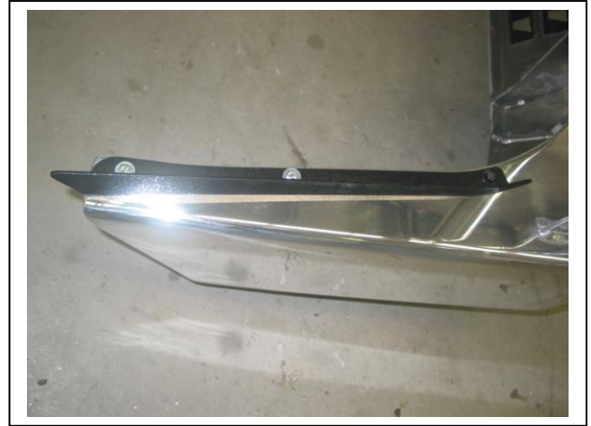
Figure 10: Install infill's to top of ECB protection bar. Paint front bolt black.
